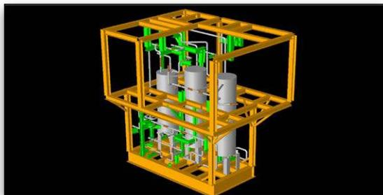
*SACS – Combined piping and structural model (secondary steel in green)*
