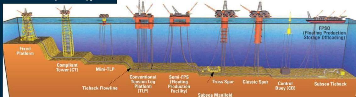
**SACS has applications for all types of offshore structures and vessels**
